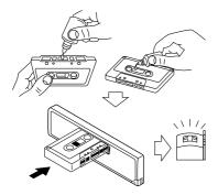
• Clean the heads after every 10 hours of use using a wet-type head cleaning tape (available at an audio store).
